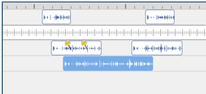
Fig. 4.18 Example of Calls Improperly Merged Because of Vox Timeout
