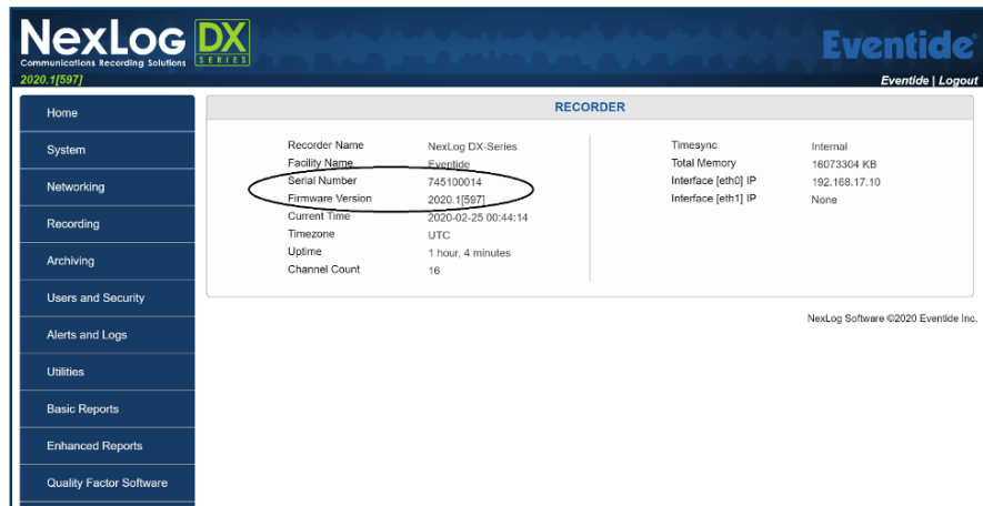
Fig. 1.4 Configuration Manager Home Screen (with Serial and Firmware circled)
