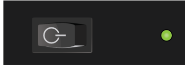
Fig. 2.5 Power Switch (Close-Up)
